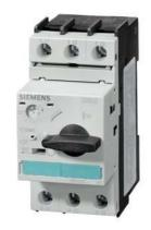
Circuit breaker size S0 for motor protection CLASS 10 A-release 7...10 A Short-circuit release 130 A Screw terminal Standard switching capacity !!! Phased-out product !!! Successor is SIRIUS 3RV2 Preferred successor type is >>3RV2011-1JA10<<
